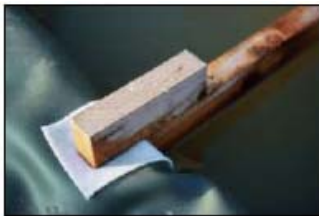
Fig.: Protective fleece functioning as a cushion
